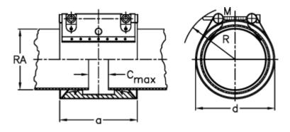
a = 98.0C max with insertion band = 25d = 110M (screw) = M10Nominal pressure (bar) = 16R = 130RA = 90.0RA min-RA max plastic = 89,0-91,0
